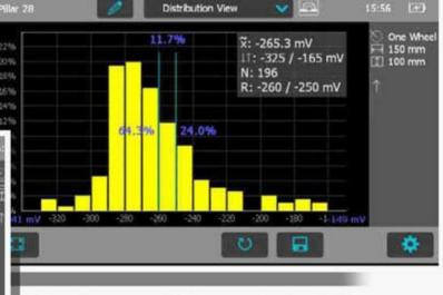
Adjustable cursors defining corrosion thresholds
